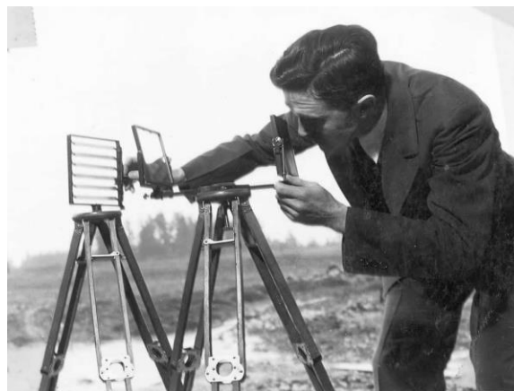
Harold Lawson from the Portland Radio Laboratory operates a heliograph, c. 1936. Heliographs were used by the Forest Service to send messages using sunlight reflected in flashes from a mirror.
